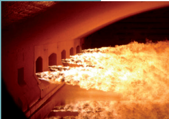
Figure 12.17. a) Oil combustion in typical float furnace today (left). b) Demonstration of viable clean hydrogen combustion for glass melting (right).
