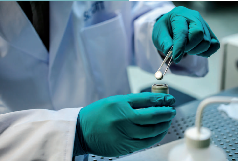
Figure 11.7. SCHOTT Glass-ceramic powder in tablet form: SCHOTT's glass ceramic powder has the potential to increase the performance and the stability of solid-state batteries for the next generation of E-Vehicles.
