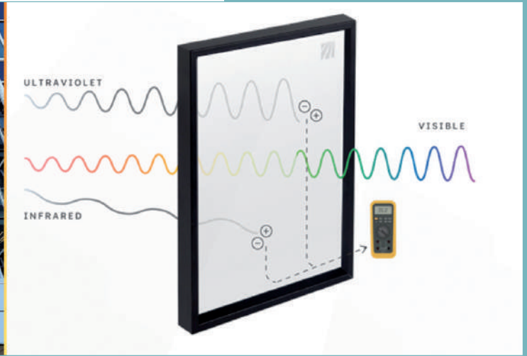
Figure 12.15. A truly transparent solar energy window introduced by Ubiquitous energy generates electricity from invisible parts of solar spectrum without diminishing visibility and aesthetic trade-off.
